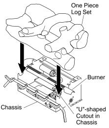
Figure 18 - Installing Heat Majic™ One-Piece Log Set
